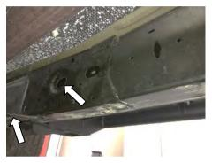
3. Fit the rubber plugs into the rear most ends of the side rails.
